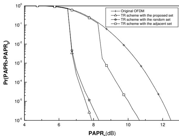
Figure 3: The CCDF of the original OFDM signal and the OFDM signal with TR scheme for various PRT sets.
