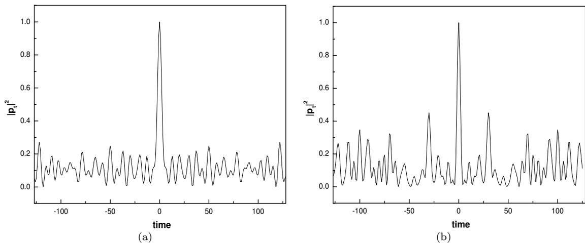
Figure 2: The power  $|p_t|^2$  of the time domain kernel (a) the proposed PRT set and (b) the random PRT set.
