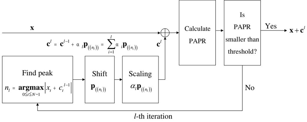
Figure 1: A block diagram of a tone reservation scheme.
