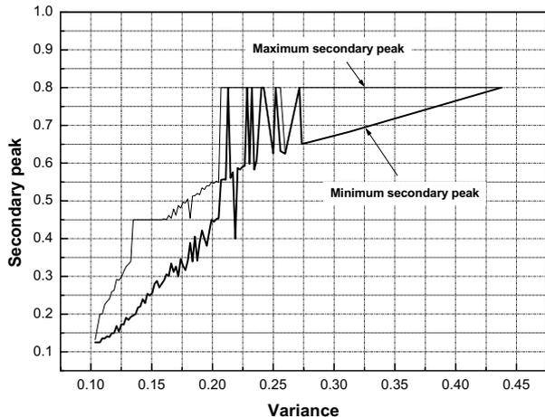
Figure 2: Relationship between the secondary peak and the variance of PRT sets when  $N = 32$  and  $W = 8$ . All possible PRT sets are used.
