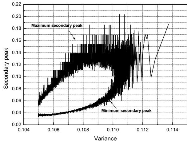
Figure 3: Relationship between the secondary peak and the variance for  $N = 1024$  and  $W = 102$ . Randomly generated  $10^7$  PRT sets are used.
