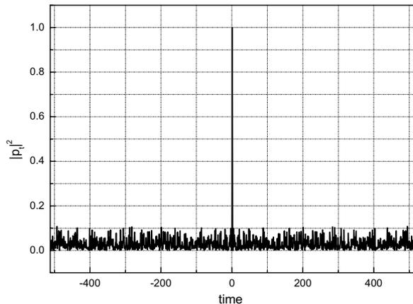
Figure 4: Power  $|p_t|^2$  of the PRT set chosen from the randomly generated  $10^7$  sets when  $N = 1024$  and  $W = 32$ .
