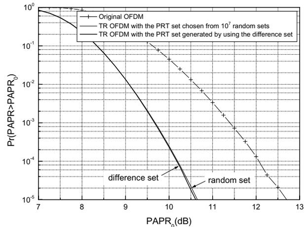
Figure 6: CCDF of the PAPR for the TR schemes with various PRT sets for  $N = 1024$  and  $W = 32$ .
