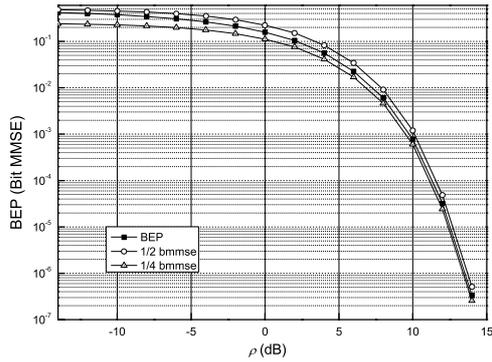
Fig. 1. The relationship between the BEP and the bit MMSE for the SISO system with binary input in the Gaussian channel.
