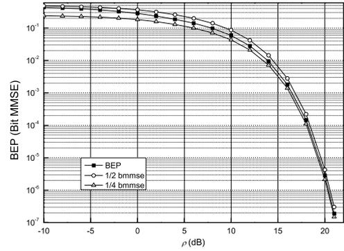
Fig. 2. The relationship between the BEP and the bit MMSE for the SISO system with Gray coded 16QAM modulation in the Gaussian channel.
