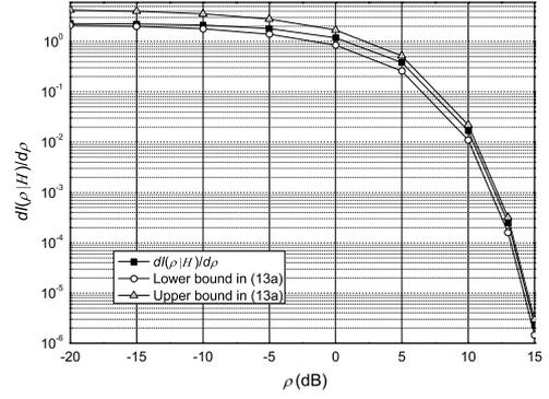
Fig. 3. The relationship between the derivative of the mutual information and the BEP for Alamouti space-time code with QPSK modulation.
