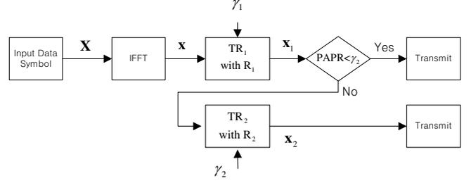
Figure 1: Block diagram of multi-stage TR scheme.
