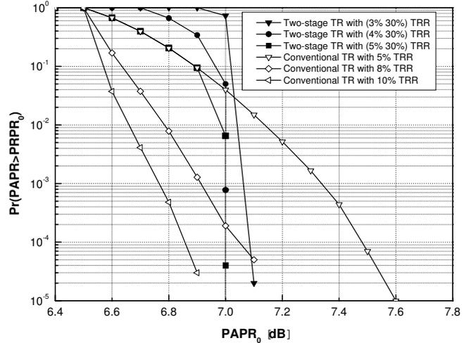
Figure 3: PAPR reduction performance of the conventional TR scheme with 5%, 8%, and 10% TRR and the multi-stage TR scheme with (3%, 30%) TRR, (4%, 30%) TRR, (5%, 30%) TRR when  $N=1024$  and 16-QAM is used.
