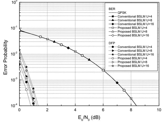
Fig. 4. Comparison of DFP and BER of the proposed BSLM and the conventional BSLM with QPSK and  $N = 256$ .
