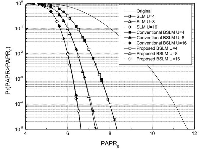
Fig. 5. Comparison of PAPR reduction performance of the proposed BSLM and the conventional BSLM with QPSK and  $N = 64$ .
