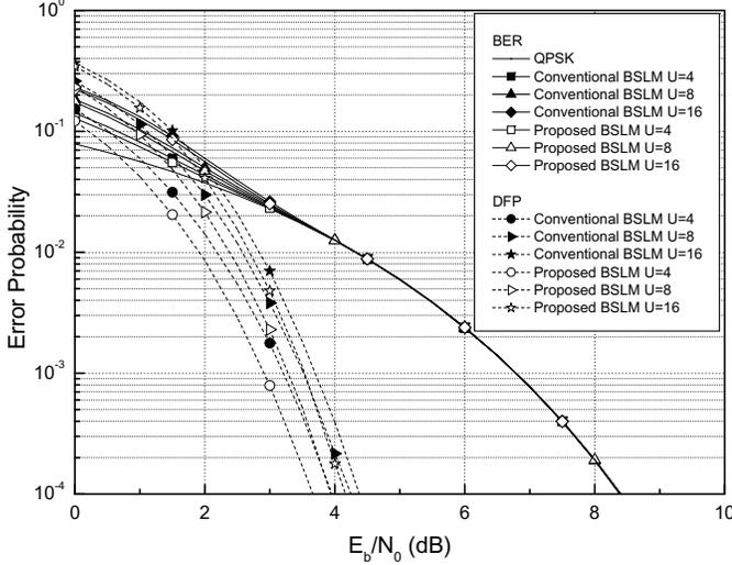
Fig. 3. Comparison of DFP and BER of the proposed BSLM and the conventional BSLM with QPSK and  $N = 64$ .
