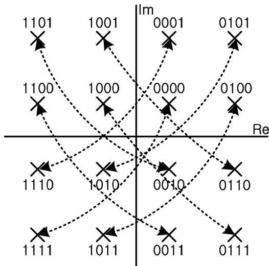
Fig. 1. An example of constellation mapping of 16-QAM with Gray mapping in PBISLM.
