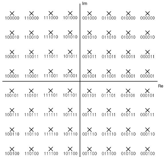
Fig. 2. An example of 64-QAM constellation with Gray mapping.
