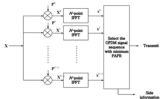
Fig. 1. A block diagram of the conventional SLM scheme.
