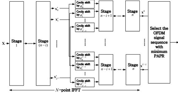
Fig. 2. A block diagram of the proposed SLM scheme ( $n = \log_2 N$ ).
