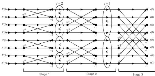
Fig. 3. Subblock partitions at stage 1 (i.e.  $i = 2$ ) and stage 2 (i.e.  $i = 1$ ) of IFFT when  $N = 8$ .
