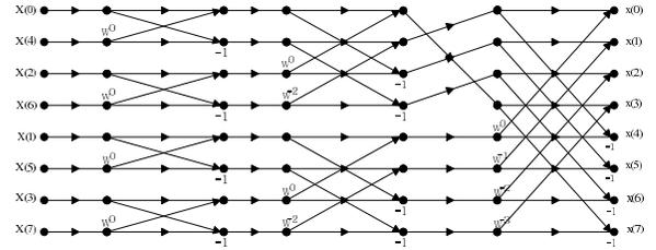
Fig. 4. An alternative OFDM signal sequence by the proposed scheme for  $N = 8$ ,  $i = 1$ , and  $a_0 = 1$  and  $a_1 = 0$ .
