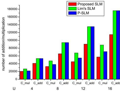
Fig. 6. Comparison of the computational complexity of the proposed SLM, P-SLM, and Lim's SLM when  $N = 2048$  and 16-QAM.
