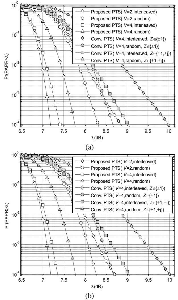
Fig. 1. Comparison of PAPR reduction performance of the conventional PTS and the proposed PTS for  $N = 512$ . (a) 16-QAM. (b) 64-QAM.
