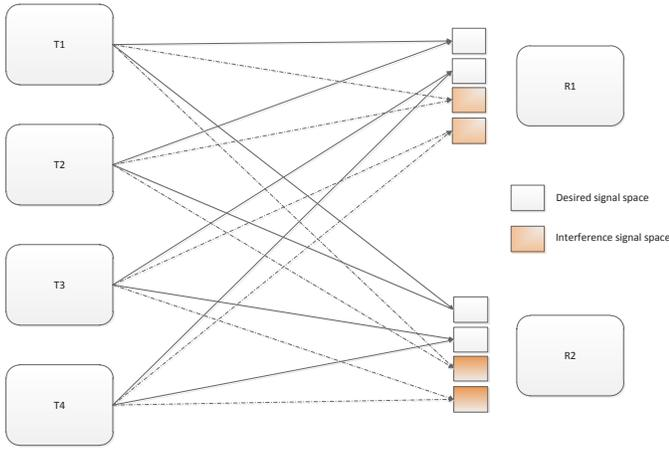
Fig. 1.  $4 \times 2$  X channel with signal and interference alignment.
