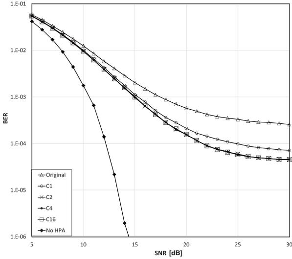
Fig. 2. BER performances of SLM schemes with CORR metric when  $N = 256$ ,  $U = 4$ , and  $L = 1, 2, 4$ , and  $16$  with  $OBO = 4$  dB.
