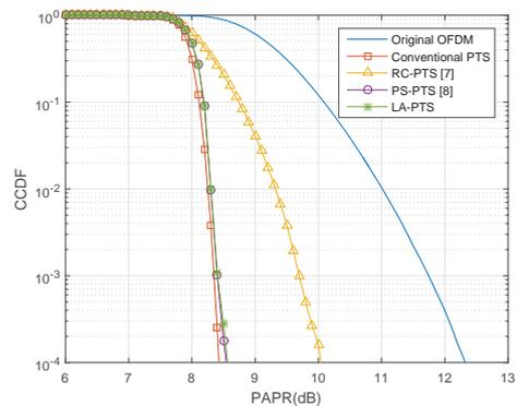
Fig. 5. Comparison of PAPR reduction performance of the conventional PTS, RC-PTS, PS-PTS, and the Proposed PTS for  $N = 1024$ ,  $L = 4$ ,  $M = 8$ ,  $W = 2$ , and  $p_\gamma = 0.07$ .
