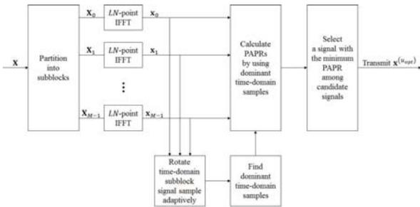
Fig. 4. A block diagram of the proposed PTS scheme.
