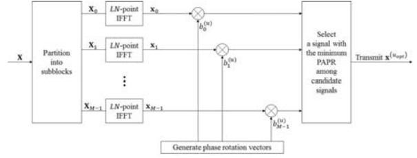
Fig. 1. A block diagram of the conventional PTS scheme.
