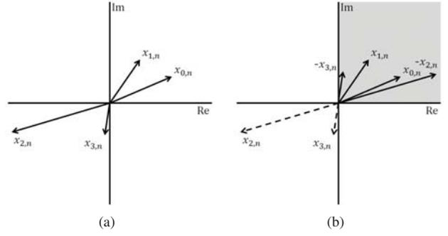
Fig. 3. The proposed method 2 for adaptive phase rotation: (a) original  $n$ -th time-domain subblock signal samples and (b) their rotation to the shaded subplane containing  $x_{0,n}$  using  $(b_{0,n}, b_{1,n}, b_{2,n}, b_{3,n}) = (1, 1, -1, -1)$  for  $M = 4$  and  $W = 2$ .
