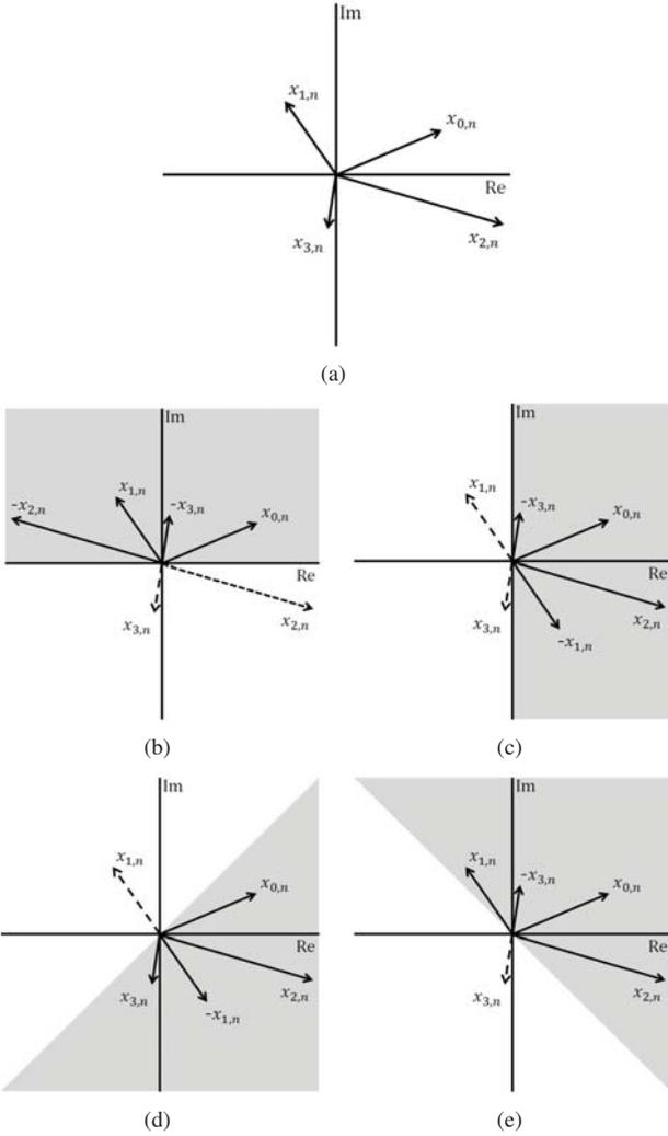
Fig. 2. The proposed method 1 for adaptive phase rotation: (a) original  $n$ -th time-domain subblock signal samples and their rotation to the shaded subplane containing  $x_{0,n}$  using  $(b_{0,n}, b_{1,n}, b_{2,n}, b_{3,n})$  (b)  $(1, 1, -1, -1)$ , (c)  $(1, -1, 1, -1)$ , (d)  $(1, -1, 1, 1)$  and (e)  $(1, 1, 1, -1)$  for  $M = 4$  and  $W = 2$ .
