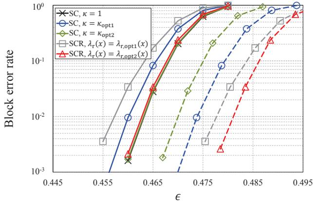
Fig. 4. Block error rate of the codes from the  $\mathcal{C}_{\text{SCm}}(3, 6, 30, 3, \kappa)$  and  $\mathcal{C}_{\text{SCRm}}(3, 6, 30, 3, \lambda_r(x))$  ensembles with  $\kappa = 1$ ,  $\kappa = \kappa_{\text{opt1}}$ ,  $\kappa = \kappa_{\text{opt2}}$ ,  $\lambda_r(x) = \lambda_{r,\text{opt1}}(x)$ , and  $\lambda_r(x) = \lambda_{r,\text{opt2}}(x)$ .
