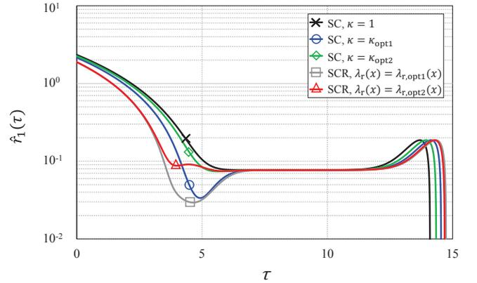
Fig. 3.  $\hat{r}_1(\tau)$  for the  $\mathcal{C}_{\text{SCM}}(3, 6, 30, 3, \kappa)$  and  $\mathcal{C}_{\text{SCR}}(3, 6, 30, 3, \lambda_r(x))$  ensembles with  $\kappa = 1$ ,  $\kappa = \kappa_{\text{opt1}}$ ,  $\kappa = \kappa_{\text{opt2}}$ ,  $\lambda_r(x) = \lambda_{r,\text{opt1}}(x)$ , and  $\lambda_r(x) = \lambda_{r,\text{opt2}}(x)$  at  $\epsilon = 0.47$ .
