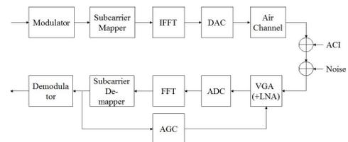
Fig. 2. Structure of AGC algorithm 2.
