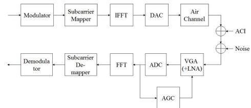
Fig. 1. A simplified system model of OFDM wireless communication system including AGC algorithm 1.
