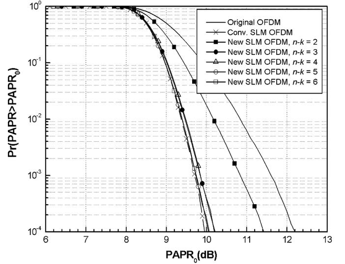
Fig. 3. CCDF of the PAPR of new and conventional SLM OFDM scheme for some stages of multiplication with phase sequences when  $N = 2048, U = 4$ , and 16-QAM constellation are used.
