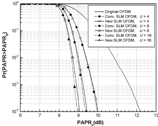
Fig. 4. Performance comparison of the conventional SLM OFDM scheme and the new SLM OFDM scheme when  $N = 2048$ ,  $n - k = 5$ , and 16-QAM constellation are used.
