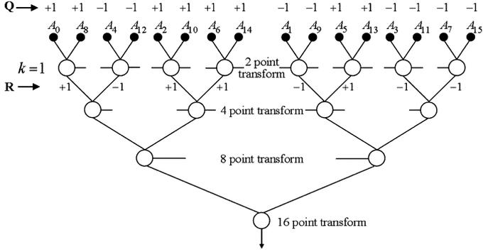
Fig. 2. Example of the phase sequence generation and the successive doubling method when  $N = 16$  and  $k = 1$  are used.
