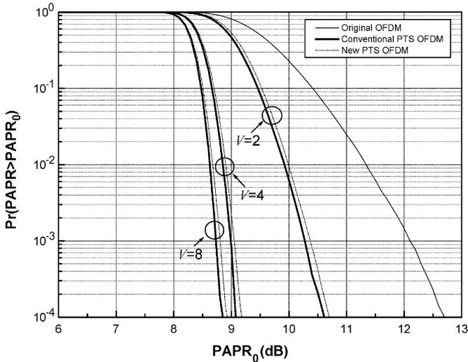
Fig. 4. PAPR reduction performance comparison of the conventional PTS OFDM scheme and the new PTS OFDM scheme when  $N = 2048$ ,  $n - l = 5$ , 16-QAM constellation, and four times oversampling are used.
