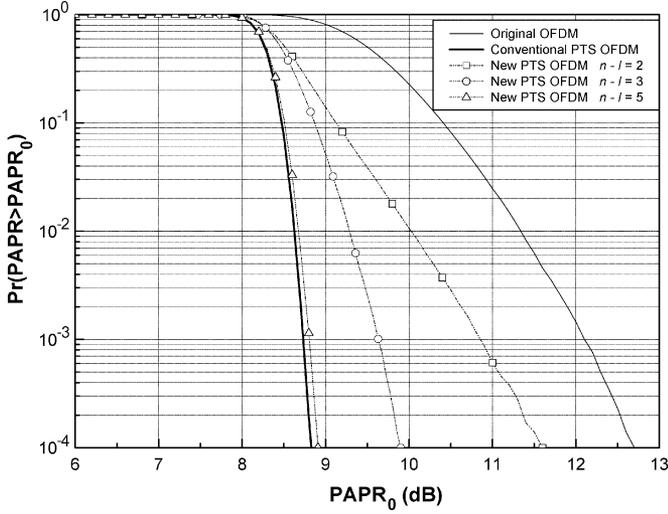
Fig. 3. CCDF of the PAPR of new and conventional PTS OFDM scheme for various stages of multiplication when  $N = 2048$ ,  $V = 8$ , 16-QAM constellation, and four times oversampling are used.
