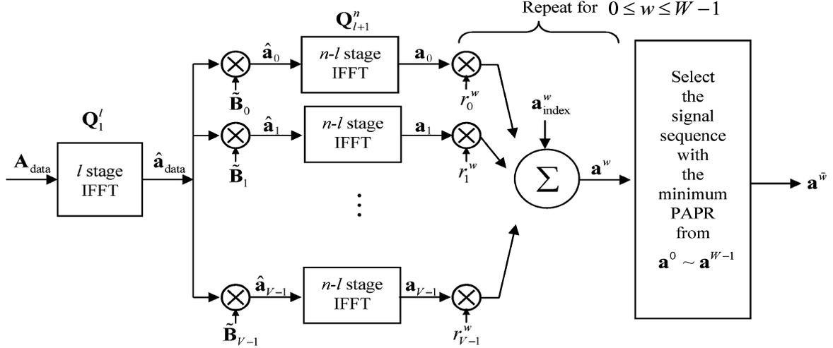
Fig. 1. Block diagram of the new PTS scheme.
