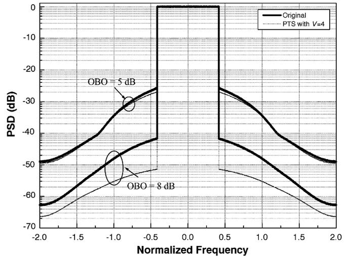
Fig. 6. PSD of the original OFDM scheme and the new PTS OFDM scheme when  $N = 2048$ ,  $n - l = 5$ , 16-QAM constellation, four times oversampling, and SSPA with  $p = 10$  are used.
