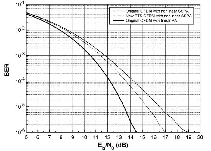
Fig. 5. AWGN channel BER performance of the original OFDM scheme and the new PTS OFDM scheme with  $N = 2048$ ,  $n - l = 5$ , 16-QAM constellation, and four times oversampling when the nonlinear SSPA with  $p = 10$  are operated at the OBO of 5 dB.
