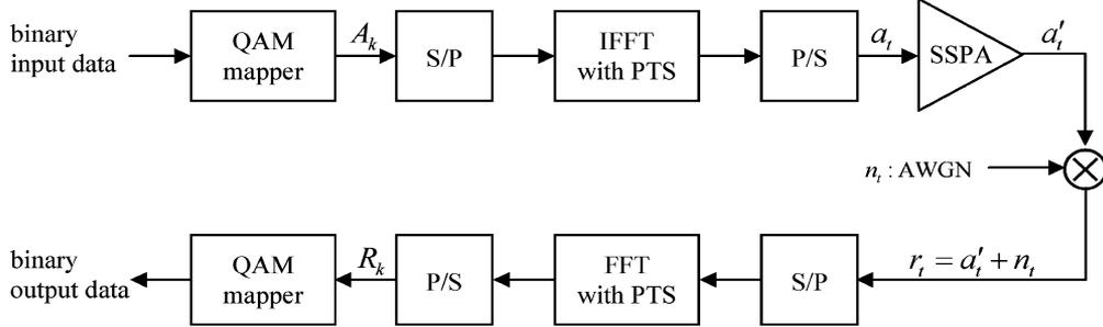
Fig. 2. A new PTS OFDM system model with SSPA and AWGN channel.
