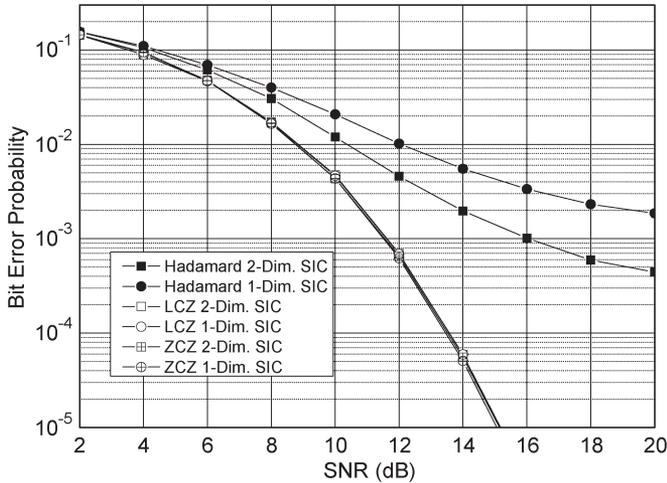
Fig. 5. Performance comparison of 2-D and 1-D SICs for  $4 \times 4$  multicode MIMO systems with QPSK when  $K = 8$  and  $L = 3$ .
