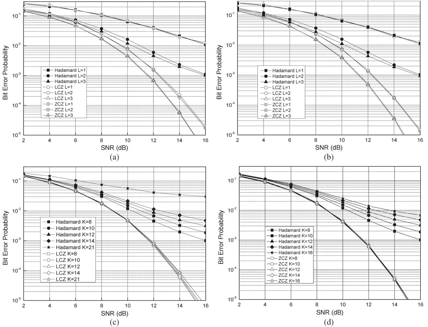
Fig. 2. Performance comparison of  $4 \times 4$  multicode MIMO systems with QPSK using 2-D SIC. (a) Various  $L$  values with  $K = 8$  under exponential power profile. (b) Various  $L$  values with  $K = 8$  under uniform power profile. (c) Various  $K$  values with  $L = 3$  for LCZ sequences under exponential power profile. (d) Various  $K$  values with  $L = 3$  for ZCZ sequences under exponential power profile.
