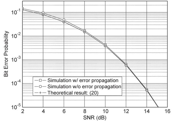
Fig. 6. Comparison of theoretical and simulation results when ZCZ sequences are used for  $4 \times 4$  multicode MIMO systems with  $K = 8$  and  $L = 3$ .
