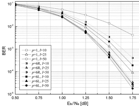
**Fig. 4** BER performance of irregular B-LDPC code of length 2304 and rate 1/2 for IEEE 802.16e using various decoding schemes and iterations with  $p = 6$ .
