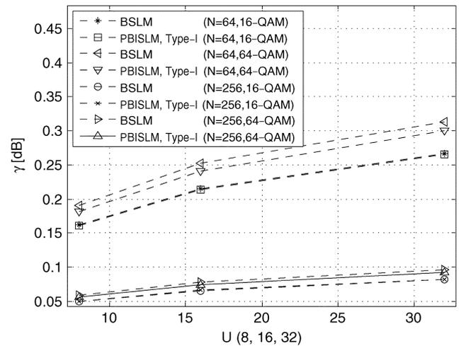
Fig. 5. Shaping gain of BSLM and PBISLM with  $N = 64$  and 256 for  $U = 8, 16,$  and 32.
