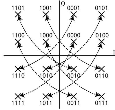
Fig. 1. An example of partial bit inversion of Gray mapped 16-QAM constellation for PBISLM.
