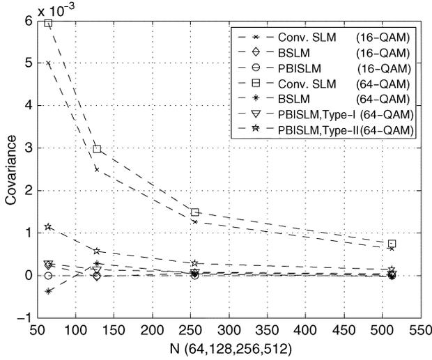
Fig. 3. Comparison of the covariance of average symbol powers of two alternative symbol sequences for various SLM schemes.
