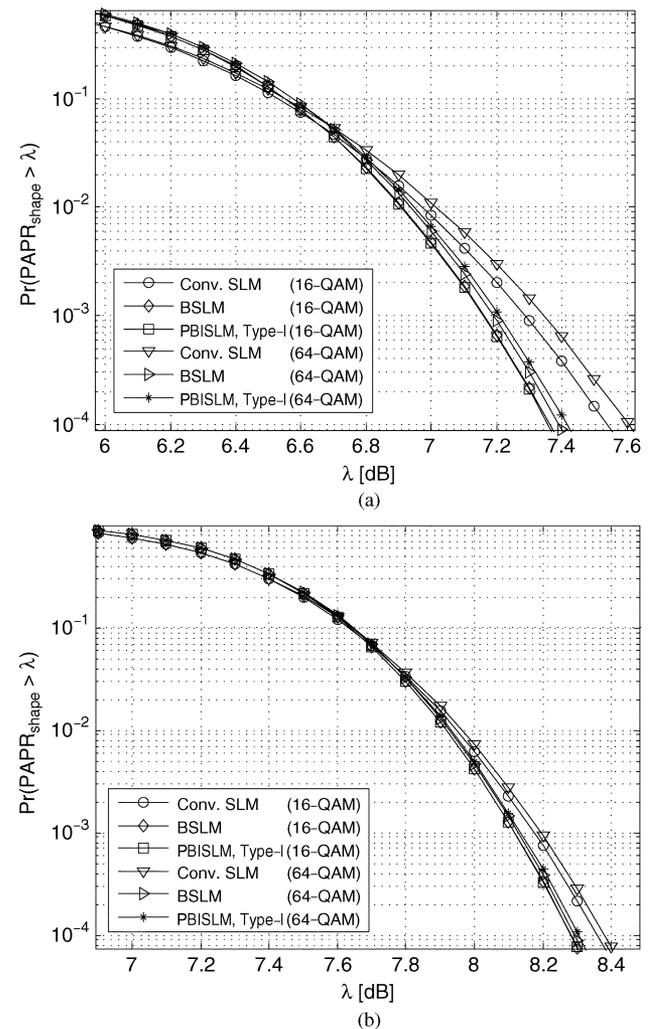
Fig. 6. Comparison of  $\text{PAPR}_{\text{shape}}$  reduction performance of the conventional SLM and proposed schemes for  $U = 16$ : (a)  $N = 64$ ; (b)  $N = 256$ .
