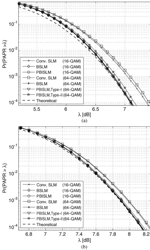
Fig. 4. Comparison of PAPR reduction performance of the conventional SLM, proposed schemes, and theoretical CCDF of (3) for  $U = 8$ : (a)  $N = 64$ ; (b)  $N = 256$ .
