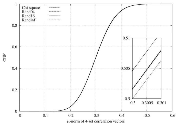
Fig. 2. Comparison between cumulative distribution of  $l_2$ -norm of 4-set correlation vectors for random sensing matrices with several alphabet size and chi-square distribution with 12 degree of freedom.
