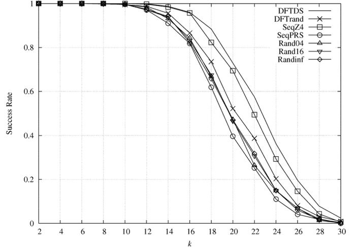
Fig. 1. Success rate of reconstruction with OMP;  $65 \times 4161$  DFT matrices,  $61 \times 3844$  PRS matrix,  $63 \times 4096$  random and family A matrices.
