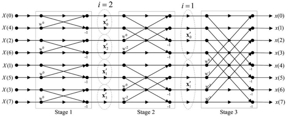
Fig. 3 Subblock partitions at stage 1 (i.e.  $i = 2$ ) and stage 2 (i.e.  $i = 1$ ) of IFFT when  $N = 8$  ( $W = e^{-j(2\pi/8)}$ )
