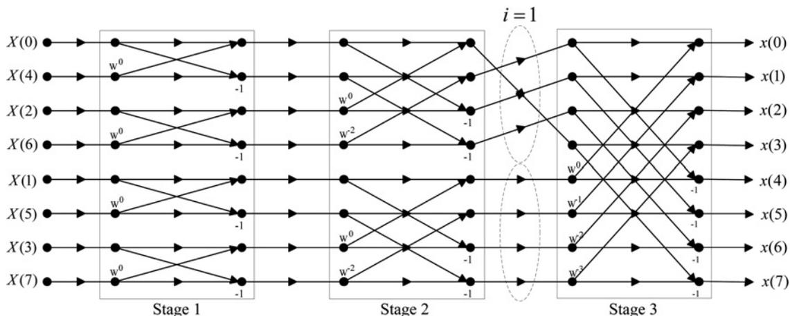
Fig. 5 Alternative OFDM signal sequence generated by the proposed scheme for  $N=8$  and  $i=1$  using  $a_0=1$  and  $a_1=0$
