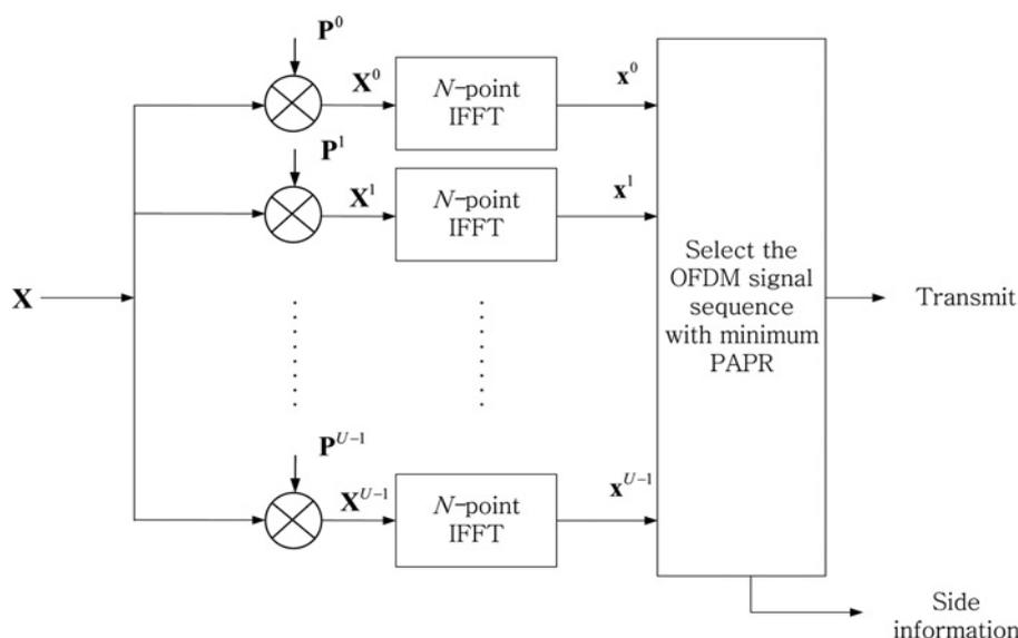
Fig. 1 Block diagram of the conventional SLM scheme
