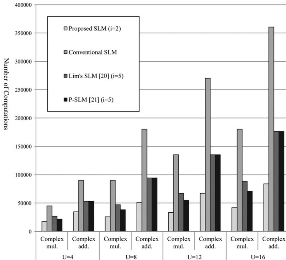
**Fig. 6** Comparison of the computational complexity of the proposed SLM, P-SLM [21], Lim's SLM [20] and the conventional SLM when  $N = 2048$
