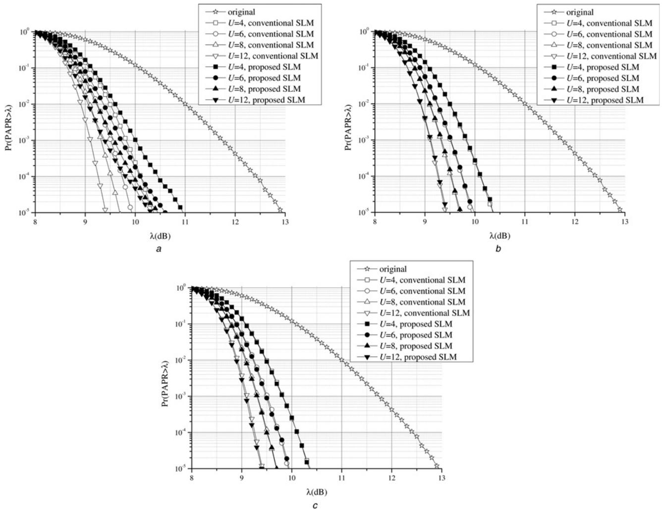
**Fig. 7** Comparison of PAPR reduction performance of the proposed and the conventional SLM schemes when  $N = 1024$  and 16-QAM and four times oversampling are used
