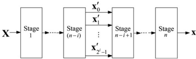
Fig. 2 Block diagram of the ordinary  $N$ -point decimation-in-frequency IFFT ( $n = \log_2 N$ )
