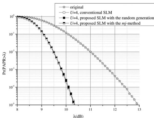
**Fig. 8** Comparison of the PAPR reduction performance of the proposed SLM scheme using the  $mj$ -method and the random generation method when  $N=1024$ ,  $U=4$ , and  $i=3$  and 16-QAM and four times oversampling are used
