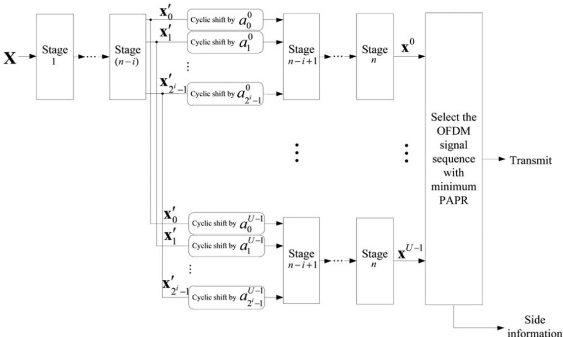
Fig. 4 Block diagram of the proposed SLM scheme ( $n = \log_2 N$ )
