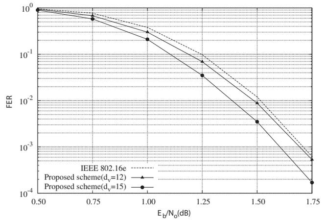
Fig. 5. Performance comparison of the QC LDPC codes with  $n=2304$  and  $R=1/2$ .
