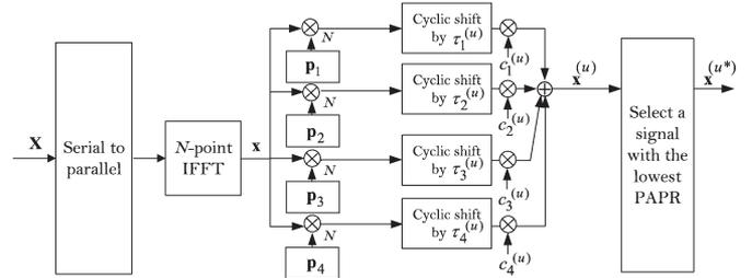
Fig. 1. A block diagram of Class-III SLM scheme.
