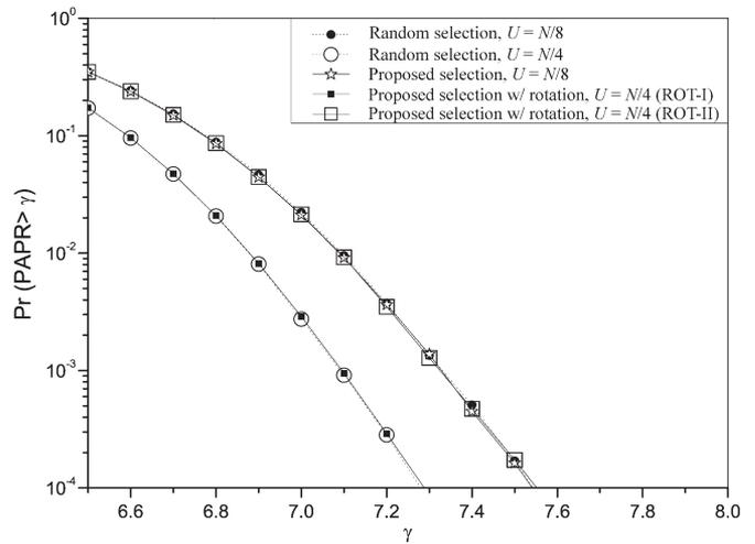
Fig. 3. Comparison of PAPR reduction performance of Class-III SLM scheme by random selection, proposed selection, ROT-I, and ROT-II when 16-QAM,  $N = 256$ , and  $U = N/8$  or  $N/4$  are used.
