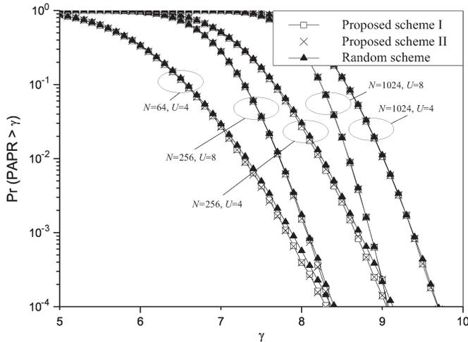
Fig. 2. Comparison of PAPR reduction performance of Class-III SLM scheme by random selection and proposed selection I and II when 16-QAM,  $N = 64, 256, 1024$ , and  $U = 4$  and  $8$  are used.
