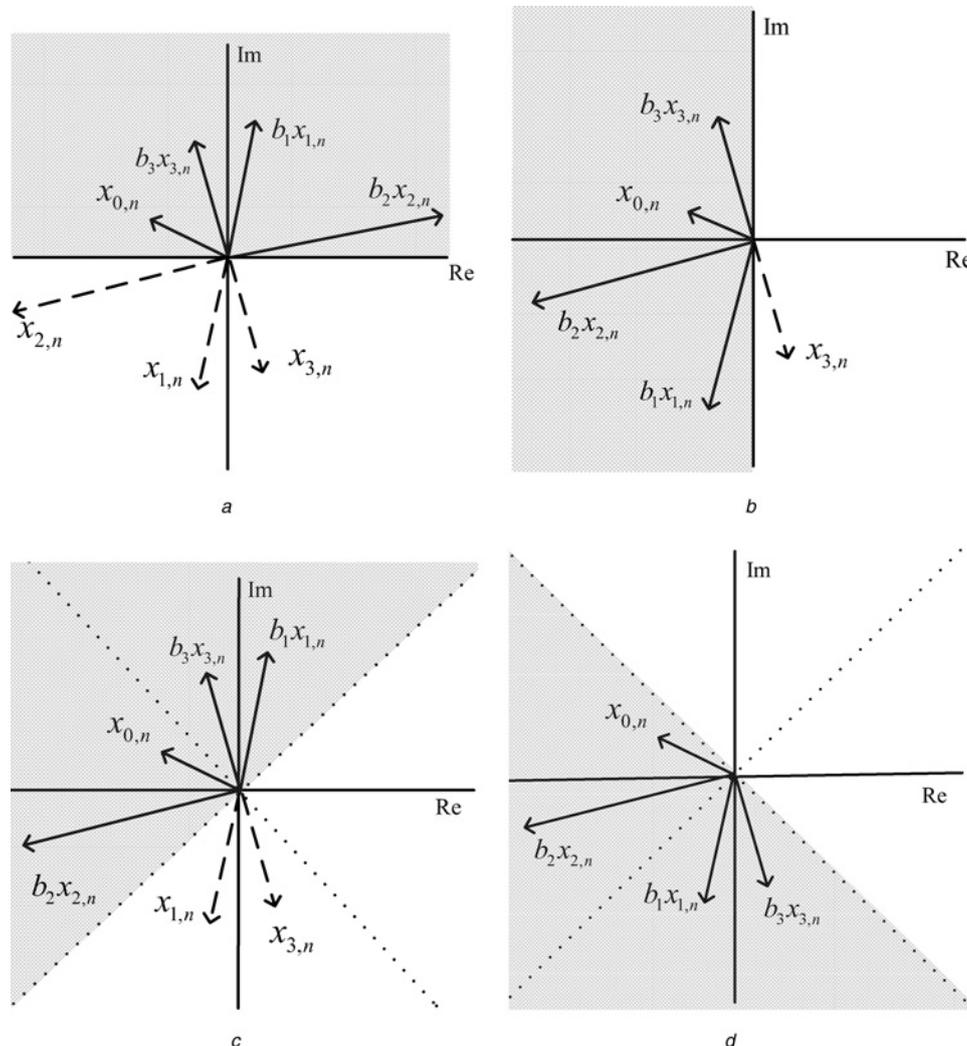
**Fig. 2** Rotation of the  $n$ th IFFTed signal samples by  $0^\circ$  or  $180^\circ$  to the shaded sub-plane containing the IFFTed signal sample  $x_{0,n}$  of the first subblock using  $(1, b_{1,n}, b_{2,n}, b_{3,n})$
