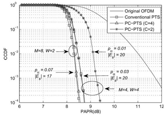
**Fig. 8** Comparison of PAPR reduction performance of the conventional PTS and two PC-PTS schemes when  $N=1024$ ,  $L=4$ , 16-QAM,  $M=4, 8$ , and  $W=2, 4$
