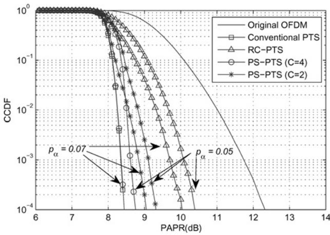
**Fig. 6** Comparison of PAPR reduction performance of the conventional PTS, RC-PTS, and PS-PTS for various  $C$  when  $N=1024$ ,  $L=4$ ,  $M=8$ ,  $W=2$ , 16-QAM, and  $p_\alpha = 0.05, 0.07$
