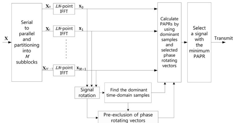
**Fig. 4** Block diagram of the proposed PTS scheme based on signal rotation and pre-exclusion
