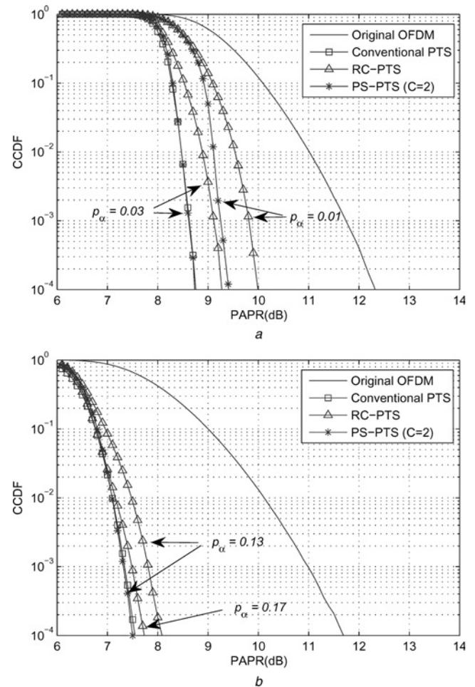
**Fig. 5** Comparison of PAPR reduction performance of the conventional PTS, RC-PTS, and PS-PTS when  $L=4$ ,  $M=4$ ,  $C=2$ ,  $W=4$  and 16-QAM
