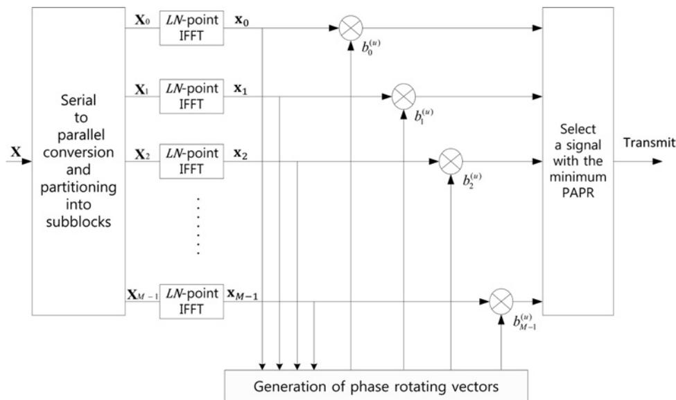
Fig. 1 Block diagram of the conventional PTS scheme
