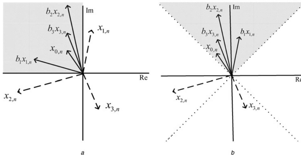
**Fig. 3** Rotation of the  $n$ th IFFTed signal samples by  $0^\circ$ ,  $90^\circ$ ,  $180^\circ$ , or  $270^\circ$  to the shaded sub-plane containing the IFFTed signal sample  $x_{0,n}$  of the first subblock using  $(1, b_{1,n}, b_{2,n}, b_{3,n})$
